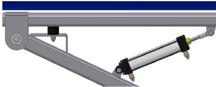
Figure 1-8. Installed Cylinder Assembly
