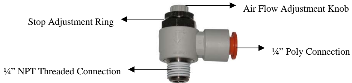
Figure 3-18. Pneumatic Flow Adjustment
