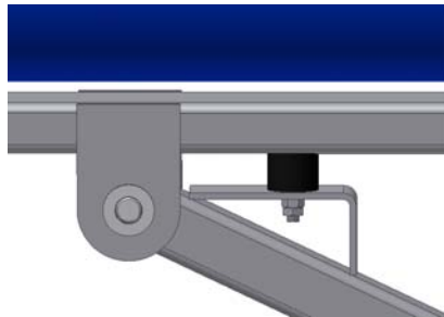
Figure 1-9. Mounted Bumper Stop
