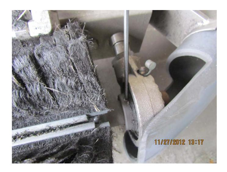
• USING 3/32 ALLEN WRENCH, REMOVE 2 BEARING COLLAR SET SCREWS FROM BEARING AT ENTRANCE END.
