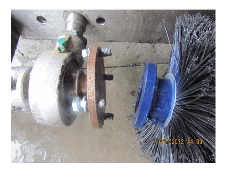
APPLY ANTI SEIZE TO BOLTS AND MOUNT EXIT & ENTRANCE END OF BRUSH TO SPINDLES.
