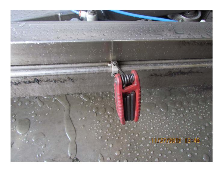
• USING A 1/8 ALLEN WRENCH, REMOVE SPLIT COLLAR SUPPORT BRACKET FROM FRAME AND REMOVE MANIFOLD PIPE.
