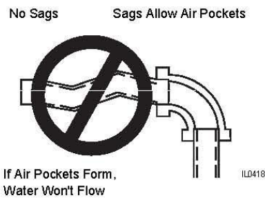
Figure 2 - No Air Pockets in Inlet Pipe
