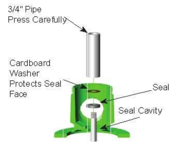
Figure 18 - If Necessary, Press With Cardboard And Pipe
