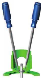
Figure 16 - Remove Mechanical Seal
