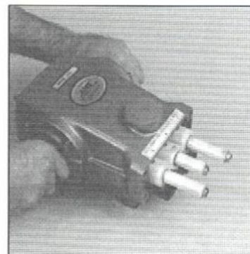
Proper Alignment of Ceramic Plungers for reassembly
