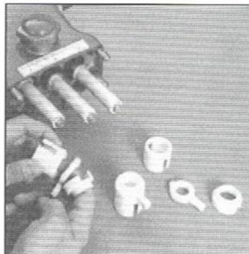
Removal of Seal Retainers and Wicks
