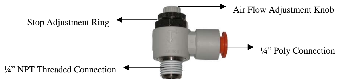
Figure 1-19. Pneumatic Flow Adjustment
