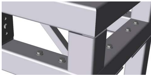
Figure 1-2. Header Assembly Bolted to Legs
