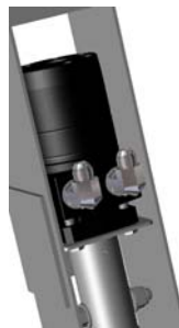
Figure 1-28. One of the Two Hydraulic Motors used for Brush Rotation on the Flex Wrap
