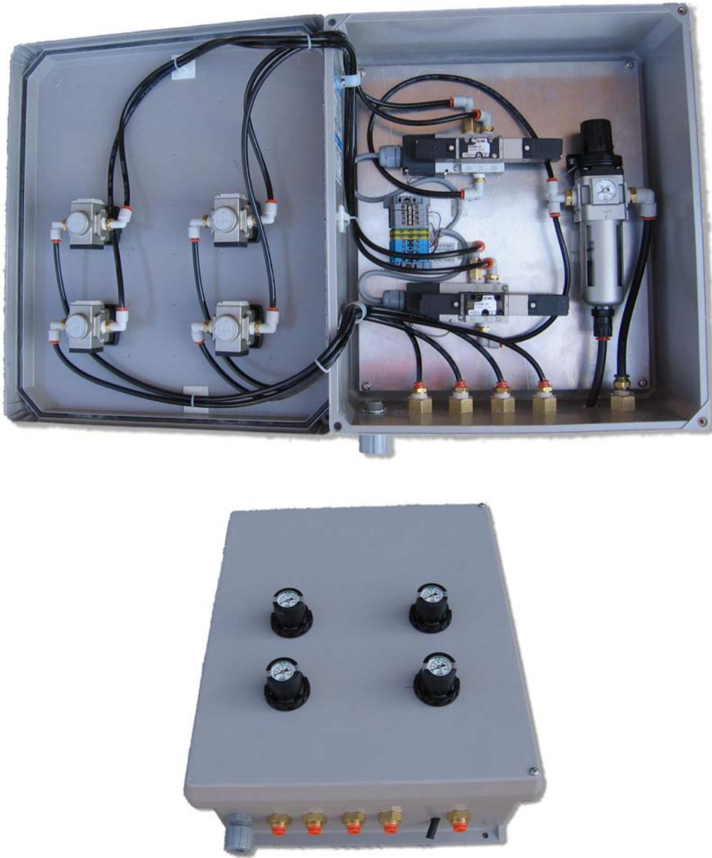
Figure 1-19. Pneumatic Control Box for the Hanna Dual Pack Flex Wrap
