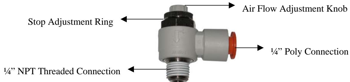
Figure 1-18. Pneumatic Flow Adjustment
