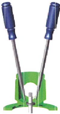
Figure 16 - Remove Mechanical Seal
