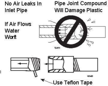
Figure 3 - Inlet Pipe Must Not Leak
