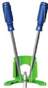
Figure 16 - Remove Mechanical Seal
