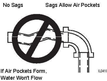
Figure 2 - No Air Pockets in Inlet Pipe
