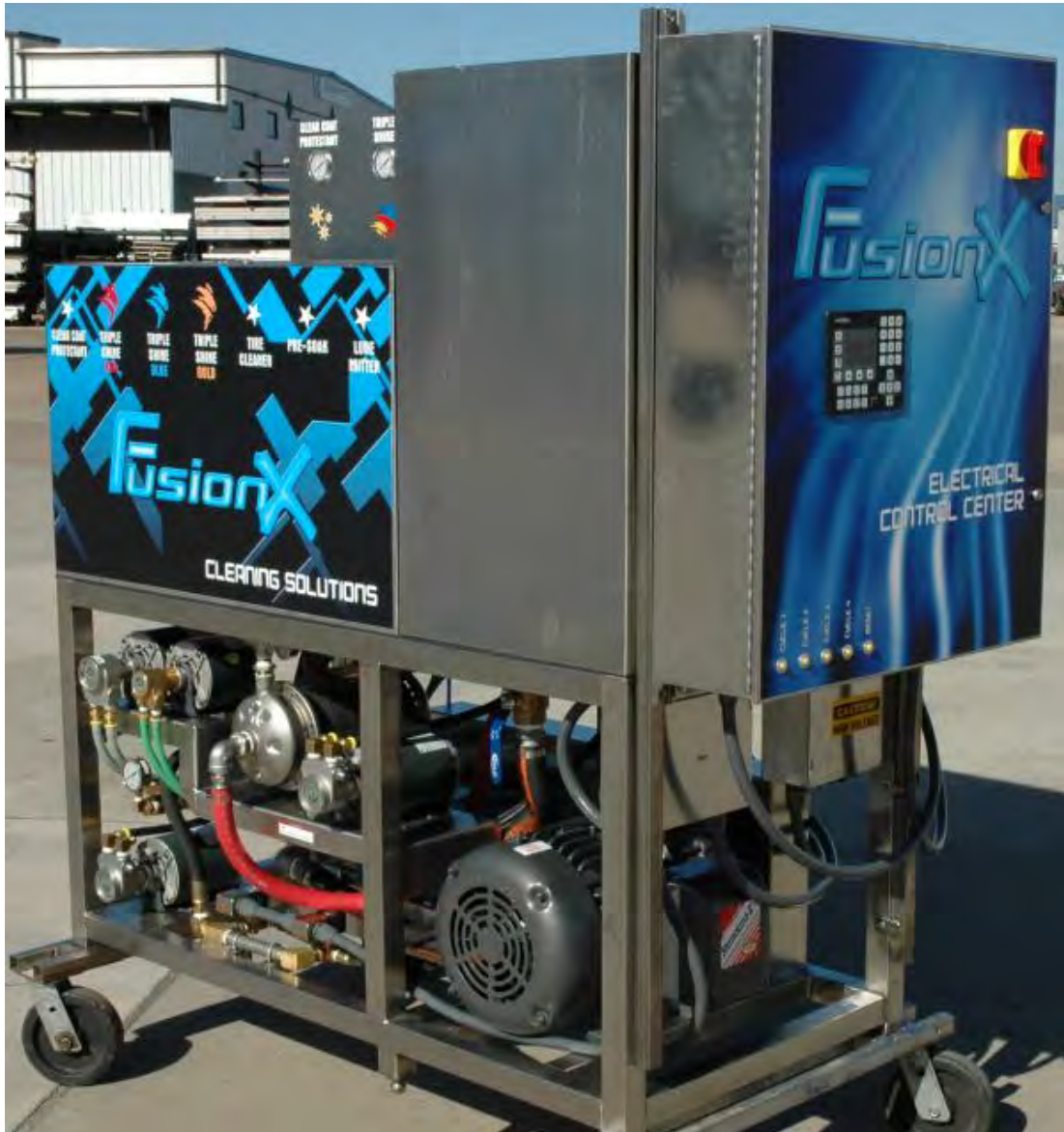
Pump Stand with Control Panel Mounted on the End
