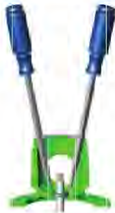
Figure 16 - Remove Mechanical Seal
