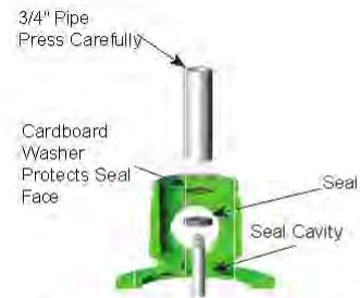
Figure 18 - If Necessary, Press With Cardboard And Pipe
